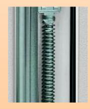
8 The spring-in-spring system on doors featuring tension spring technology ensures that a broken spring cannot be catapulted into the air and possibly cause someone injury. (B) EN 12604 ).
