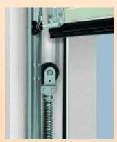
2 Anti-fall safeguard also with tension spring system The single or double spring-inspring system (2 or 4 springs) and the double steel cable arrangement on each side hold the door leaf of EcoClassic / EcoTherm doors up to 3 m wide safely in position. If a spring should break or a cable snap, simply an admissible imbalance of less than 200 N at the main closing edge is produced. (EN 12604).
